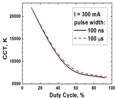
Fig.1. CCT vs. Duty Cycle of the white LED measured in the integration sphere at 100 ns and 100  $\mu$ s pulse durations.
