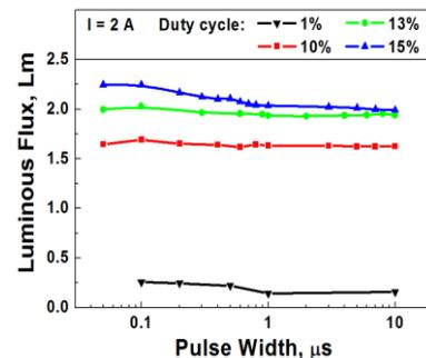
Fig. 3. Luminous flux vs. pulse width measured at different Duty cycles at 2A driving current. The figure demonstrates a possibility to keep the luminous flux independent from pulse width in the range of more than two orders.
