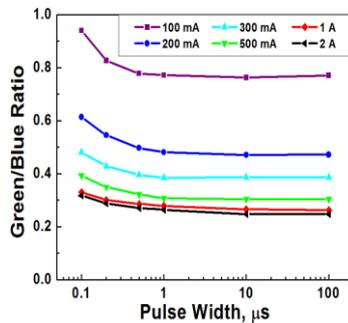
Fig.2. Green/Blue bands ratio vs. pulse width measured at different currents and 1% Duty cycle. The figure demonstrates colour mixing tunability even at non-overheated mode.
