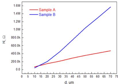
Fig. 4. Transfer resistance vs. contact pad distance of samples A, B.
