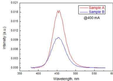
Fig 2. Electroluminescence vs. wavelength of samples A, B.
