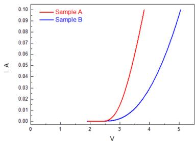
Fig 1. Current-voltage characteristics of samples A, B.
