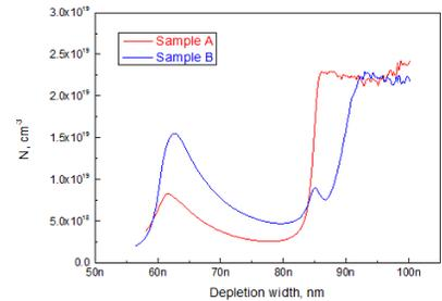
Fig 3. Charge concentration in depletion region of samples A, B.
