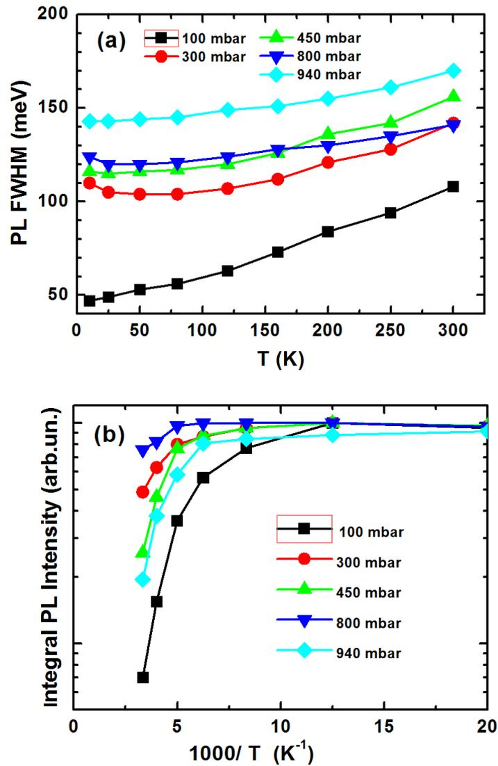
Fig. 2. Temperature dependencies of the FWHM (a) and Arrhenius plot of the PL intensity (b) obtained for the samples grown at different pressures in the Aixtron epi-system.
