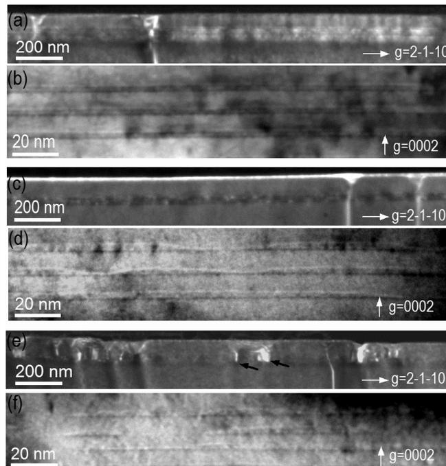
Fig.3. Cross-sectional (01-10) weak beam dark field images taken with  $g=2-1-10$  (a), (c), (e) and dark field underfocused images taken with  $g=0002$  (b), (d), (f) of the active region of the
