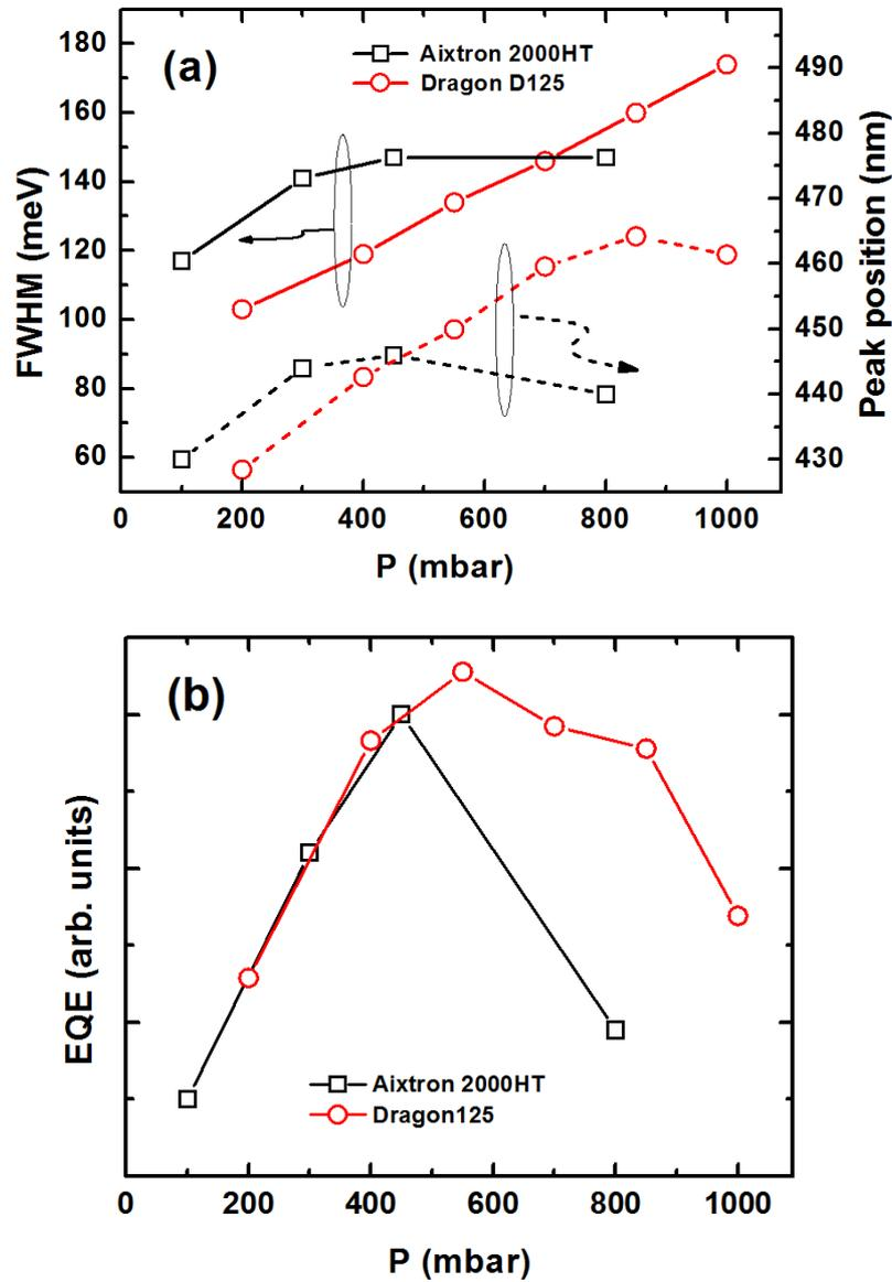
Fig. 6. EL spectrum FWHM and peak position (a) and EQE of LED structures grown in different systems: Aixtron 2000HT and Dragon 125 (b) as function of QW growth pressure.
