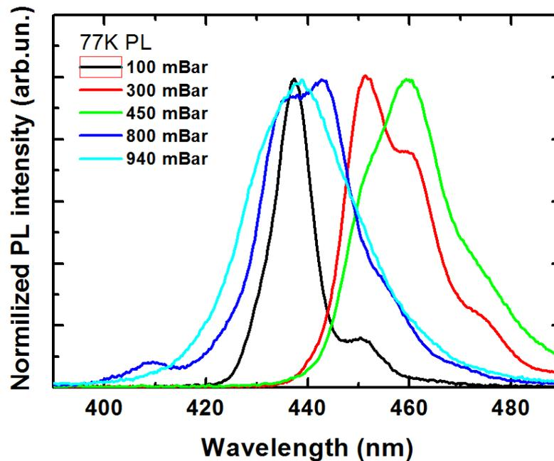
Fig. 1. PL spectra of the samples grown at different pressures in the Aixtron epi-system. An excitation wavelength is 325 nm and a current density is 20 W/cm<sup>2</sup>.
