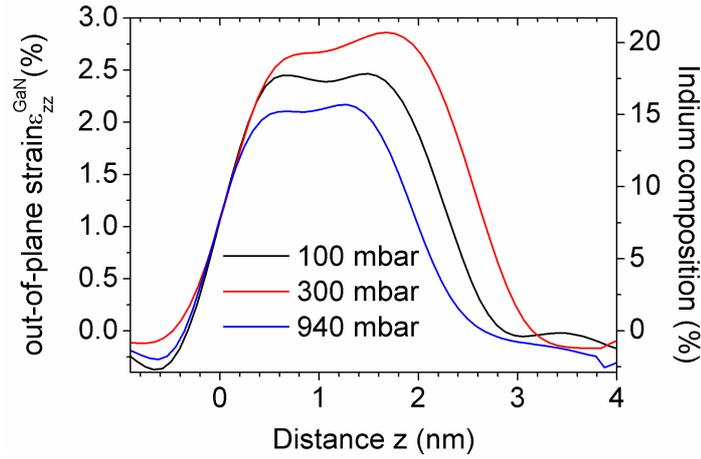
Fig. 5 Out-of-plane strain  $\varepsilon_{zz}^{\text{GaN}}$  profiles across an “average” QW grown at pressure of 100 mbar (black line), 300 mbar (red line) and 940 mbar (blue line). The right axis corresponds to indium composition within the QWs calculated from  $\varepsilon_{zz}^{\text{GaN}}$  values being corrected for a thin foil relaxation effect.
