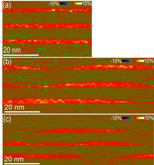
Fig. 4 Map of the out-of-plane strain relative to GaN,  $\varepsilon_{zz}^{\text{GaN}}$  obtained by geometric phase analysis of HRTEM images with a spatial resolution of 1 nm in the active region of the structures containing QWs grown at different pressures of: (a) 100 mbar; (b) 300 mbar; (c) 940 mbar.
