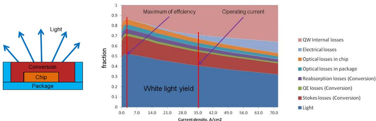
FIG. 2: Analysis of the efficiency of a white LED, where the main losses are found to be in epitaxy and conversion efficiency [8].
