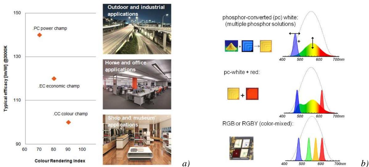
FIG. 1: a) For specific SSL applications, such as outdoor, home and/or shop illumination, typical efficacies in lm/W are plotted versus the typical CRI values. b) Description of white light generation by phosphor converted (pc) solution and by combination of LEDs emitting at different wavelengths.
