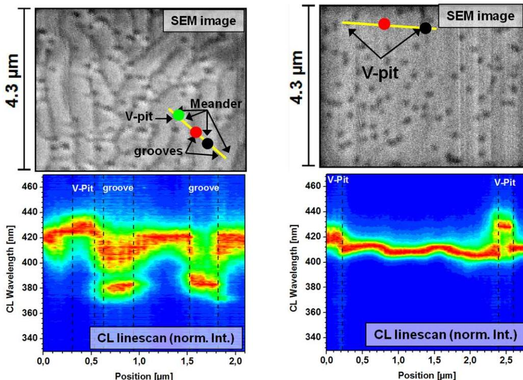
FIG. 3: The SE image (top) shows the spatial origin of the spectral line scan (dashed line) taken by cathodoluminescence (bottom) for the fast grown sample with growth rate of 433nm/h (left) and for the very slowly grown InGaN bulk layer by 133nm/h (right).
