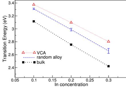
Fig. 2. Ground state transition energy resulting from VCA and random alloy based calculations. The bulk band gap is given for comparison.
