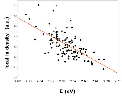
Fig. 4. Correlation between effective local In concentration and transition energy.
