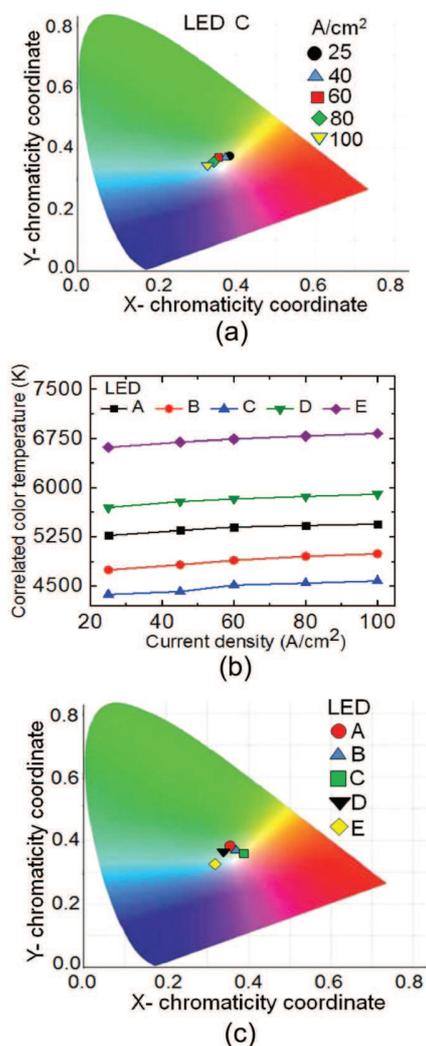
FIG. 3. (a) Trend of chromaticity coordinates of white light emission from device C with variation of injection current density; (b) variation of correlated color temperature of white light emission with injection current density for different LEDs. Solid lines are guides to the eye; (c) chromaticity coordinates of emission for different wavelength converter quantum dot white LEDs at a constant current density of 45 A/cm<sup>2</sup>.
