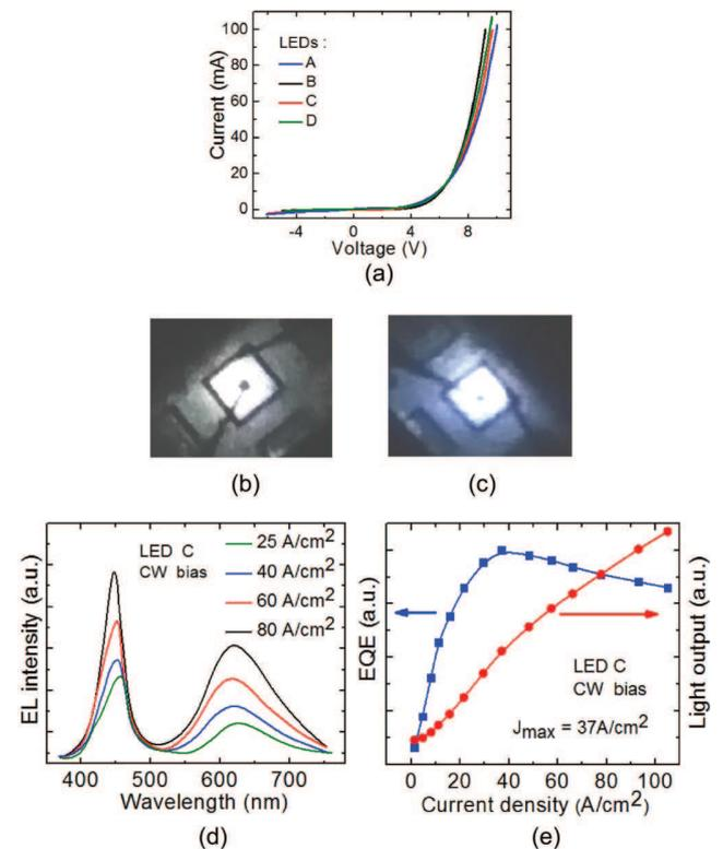
FIG. 2. (a) Measured current-voltage characteristics of white LEDs; optical micrographs of the devices biased at  $45 \text{ A/cm}^2$ : device C (b) and device E (c); (d) electroluminescence of device C as a function of injection current density; (e) light-current characteristics and external quantum efficiency of device C under CW biasing.
